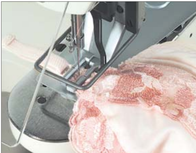
● Attaching the shoulder straps to brassier (F type)
