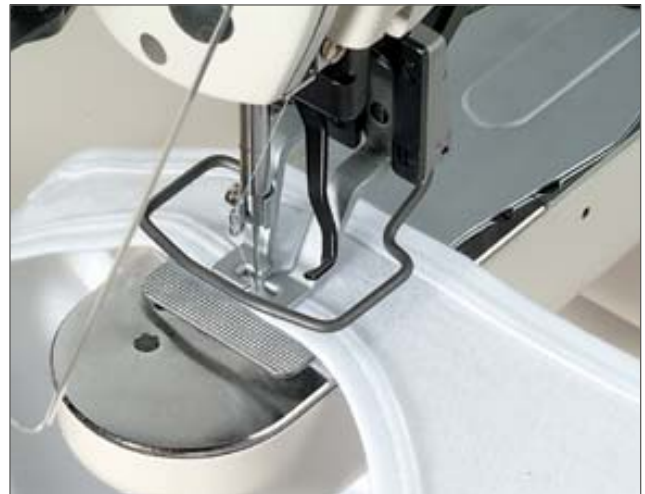
● Bartacking shoulder of running shirt (M type)
