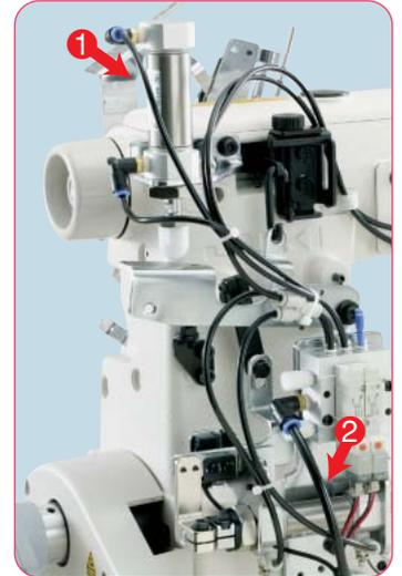
① Presser lifter drive mechanism
