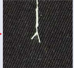
\* For the seam samples shown in the above pictures, the machine performed reverse stitching.
