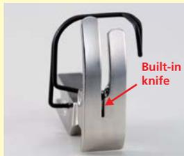
\*Needle thread waste produced by the trimming action is sucked in the clamp and automatically put into the dust bag.
