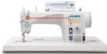
· The needle bar and thread take-up components are lubricated with the minimum required quantity of oil.
