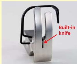
\*Needle thread waste produced by the trimming action is sucked in the clamp and automatically put into the dust bag.
