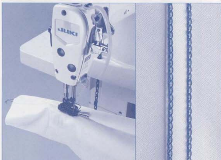
Wrong side of double chainstitch seam.
