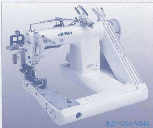
● Beautifully-finished seams are produced by smoothly feeding the overlapped parts of heavy-weight material.
