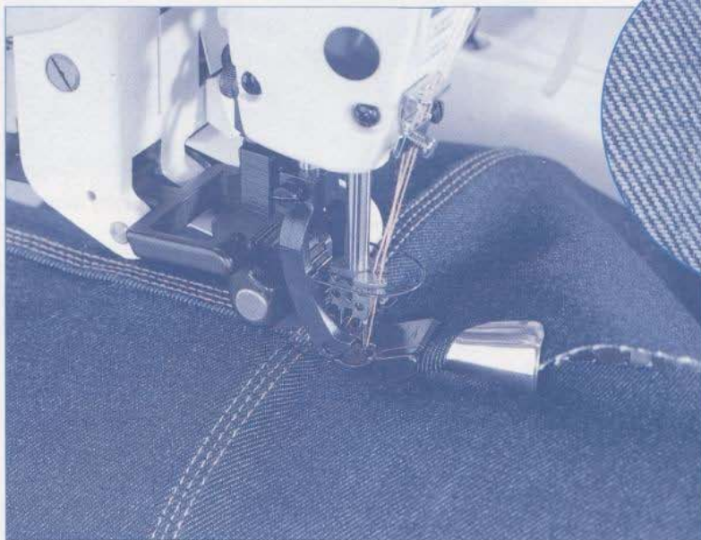
● Beautifully-finished seams are produced by smoothly feeding the overlapped parts of heavy-weight material.
