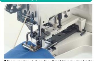
For sewing shank buttons: The thread-fray-prevention function (thread-fray-prevention function) is applicable.
