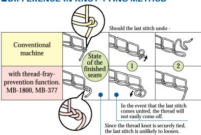
The quality of the seams was verified in the laundry test: After 200 repeated machine washings seams came untied 0 (zero) times.
