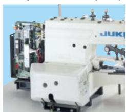
Circuit board, motor, and operation panel integrated into the machine head
