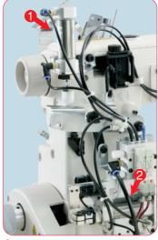
Presser lifter drive mechanism 2 Thread trimmer drive mechanism
