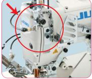
The needle thread tightening mechanism helps produce well-tensed seams even when the machine performs short stitching.
